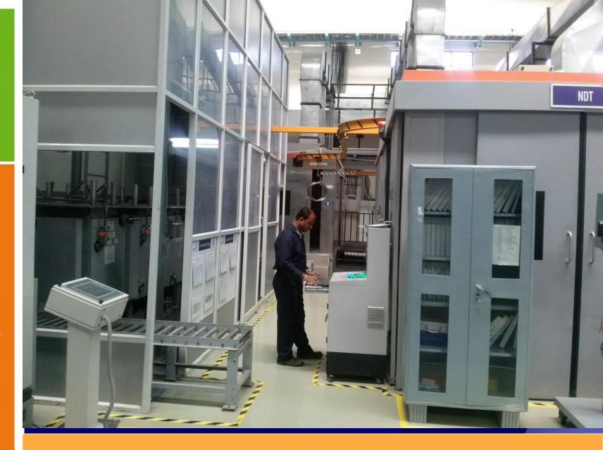
FPI FACILITY ALONG WITH PRE-CLEANING AND ELECTROSTATIC PENETRANT SPRAY TYPE FPI LINE
