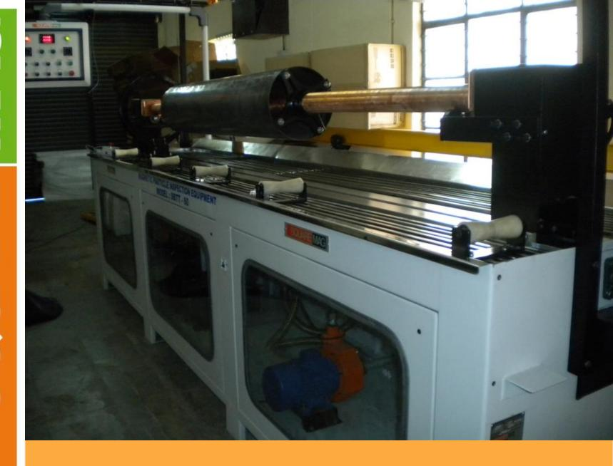
MAGNETIC PARTICLE INSPECTION SYSTEM FOR TESTING OF THIN PIPES.
